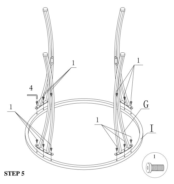
Attach table legs (G) to top frame (I) with hex socket head bolts (1). Use Allen key (4) to install bolts.
